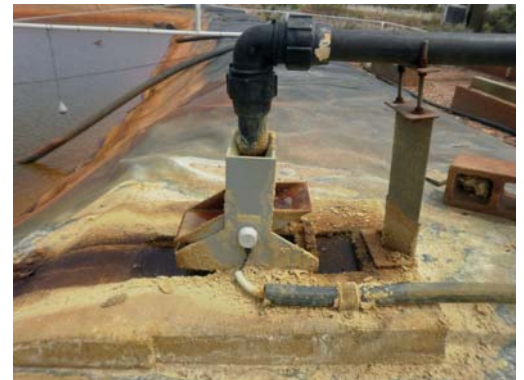
Tipping Bucket Flow Gauge Model TB1L or TB0.5L in field of use
