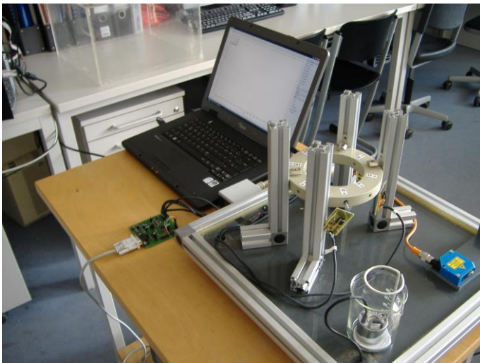
Figure 5: First experimental set-up for producing fog and measuring the scattered light with detectors mounted in ring element.
